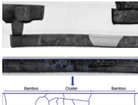
FIG.2A Void growth during electromigration
